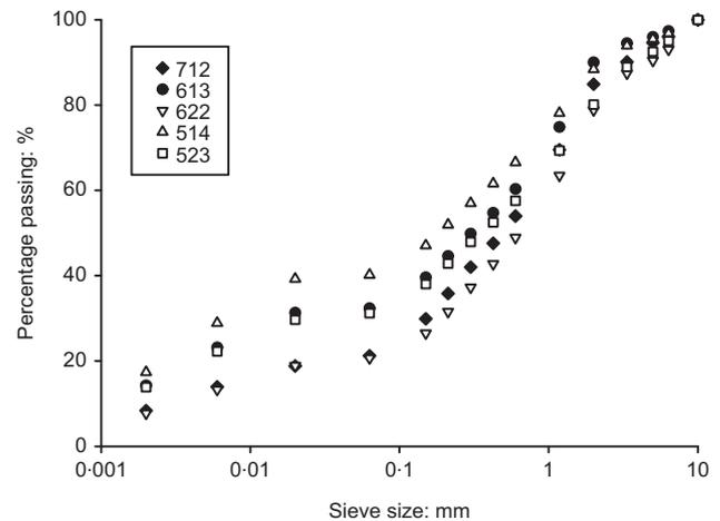
Figure 1. Particle grading curves for all RE mixes
