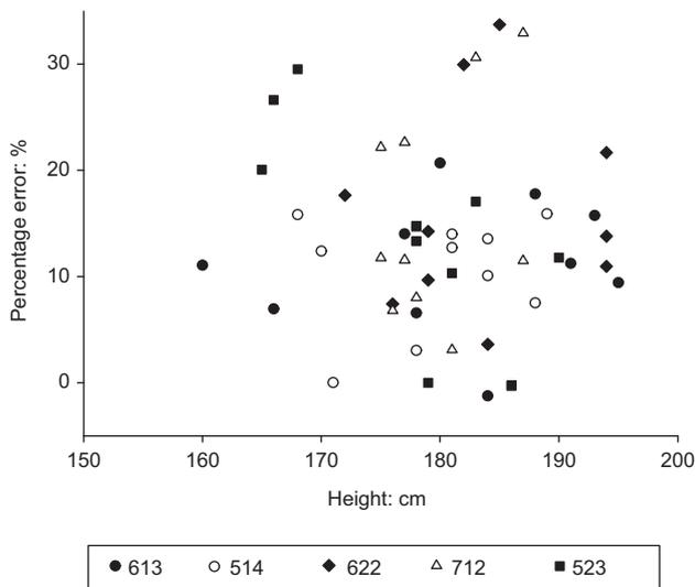
Figure 6. Percentage error plotted against height of the operator for all five RE mixes for the DT. A negative percentage error indicates a  $w$  lower than the OSET range for the given RE mix; a positive percentage error indicates a  $w$  greater than the OSET range for the given RE mix
