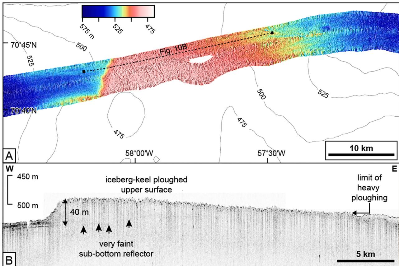
**Fig. 10.** The mid-shelf area of the Uummannaq system (located in Fig. 1). (A) Swath-bathymetric imagery showing a shallower area about 490 m deep, with deeper areas of the cross-shelf trough to west and east. (B) TOPAS shallow-acoustic profile showing a 40 m-high scarp and a highly irregular sea floor in the shallower water less than about 510 m deep.
