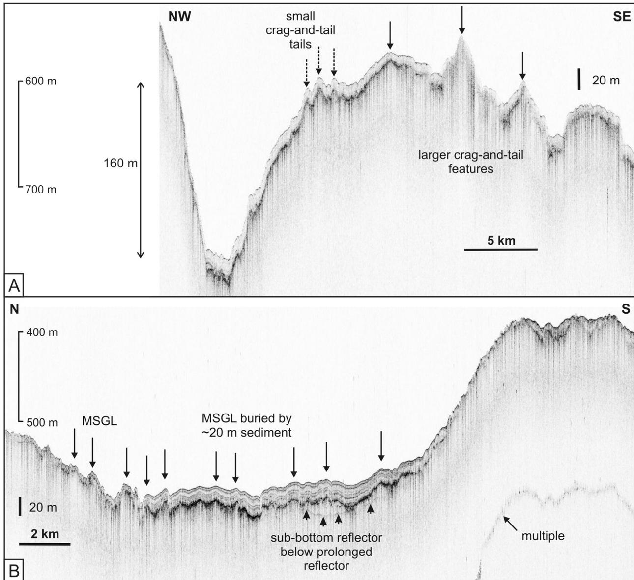
**Fig. 6.** TOPAS shallow-acoustic profiles from the outer fjord and inner shelf of the Uummannaq system (located in Fig. 8A). (A) Transect across streamlined submarine landforms in the outer fjord at 53°W. (B) Transect across the inner shelf at 55°W including the cross-shelf trough floor with streamlined sedimentary landforms, and shallower bank to the south.
