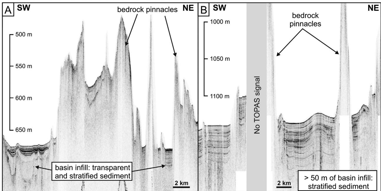
**Fig. 5.** TOPAS shallow-acoustic profiles along the axis of the inner fjord of the Uummannaq system (located in Fig. 7A). (A) From Karrat Isfjord, between 62 and 85 km from the margin of Rink Isbrae. (B) From Rink Fjord, between 10 and 30 km from the margin of Rink Isbrae.
