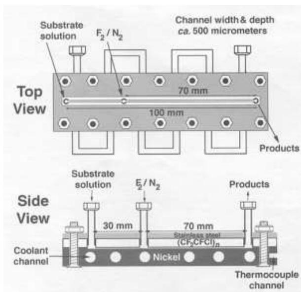
Figure 1. Single channel continuous flow device for direct fluorination processes
