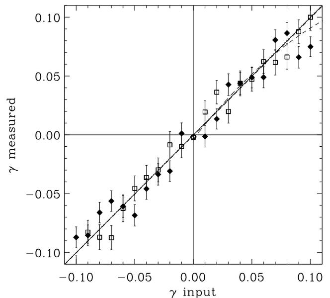
FIG. 14.—Calibration of the RRG shear measurement method from simulated COSMOS images containing a known input shear. The measured shear on the  $y$ -axis includes the shear calibration factor  $C$ . Squares: Measurements of  $\gamma_1$ . Diamonds: Measurements of  $\gamma_2$ . Solid line: Linear fit to deviations from the ideal case of  $\gamma_{\text{measured}} = \gamma_{\text{input}}$  for all points. Dashed line: Quadratic fit demonstrating that the curvature terms are negligible.
