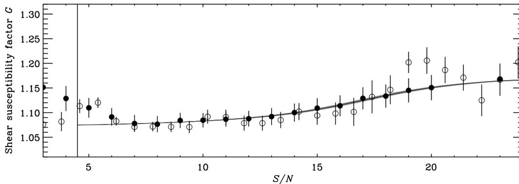
FIG. 13.—Interpolation of the shear susceptibility factor  $G$ . The filled circles show  $G$ , calculated in bins of  $S/N$ , for the COSMOS data. The open circles show the same for the simulated COSMOS images. The solid line shows the shear susceptibility model adopted for the data.
