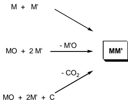
**Scheme 1** General ball milling routes to alloys.
