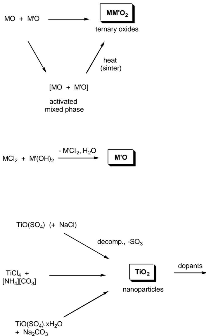
**Scheme 2** General ball milling routes to metal oxides.
