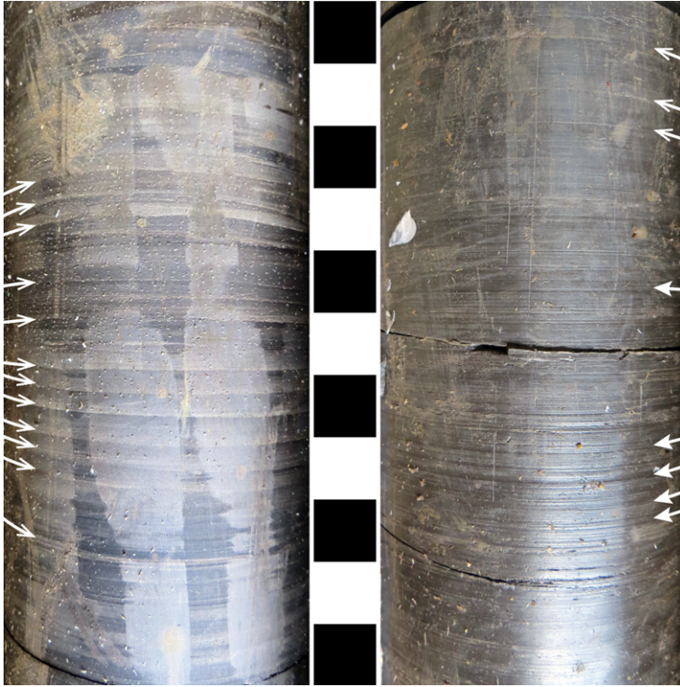
Fig. 2. Stratification in Toarcian black shales from two intervals of a core through the Whitby Mudstone Formation, Whitby, North Yorkshire (UK). Squares with an area of 1 \text{ cm}^2 each are included for scale. The arrows with an open arrowhead indicate a few prominent bedding planes, whereas the closed arrowheads point to examples of lamination planes. The most obvious bedding planes are those which are materialized by either an erosional surface with relief or a silt lag above it (left image, third arrow from above, for example). Other bedding planes are subtler (left image, fourth arrow from above, for example). All beds in the left image are thinner than 10 mm, and most are thinner than 5 mm, which would make them fall under the definition of laminae sensu McKee & Weir (1953). The interval shown in the right image is laminated, particularly the lower two-thirds shown. Bedding planes in the right image are subtler than in the left image due to reduced textural contrast between thin beds. Individual laminae are in general thinner than 1 mm. Unlike beds, laminae lack abrupt changes in texture and evidence for erosion at the stratification plane. Although the processes and environmental conditions behind their development are clearly different, McKee & Weir's descriptive terminology does not distinguish the true laminae sensu (Campbell 1967) in the right image from the 'laminae' in the left image.
