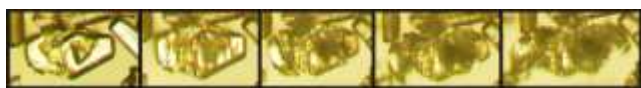
Figure 6 Photo micrographs of the dehydration of DTS tetrahydrate upon heating. The first micrograph is taken at 74 °C with the following images taken every 5 seconds at a heating rate of 10 °C min -1 .
