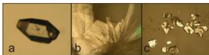
Figure 1. Photo micrographs of the diatrizoic acid hydrated crystal forms: a) DTA dihydrate, b) DTS tetrahydrate initial blades and c) DTS tetrahydrate final blocks.
