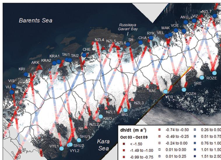
**Fig. 8.** Rate of elevation change along ICESat laser altimetry tracks for the period October 2003–October 2009. Data provided by G. Moholdt (Moholdt and others, 2012). Study glaciers are symbolized according to coast and terminus type as follows: Barents Sea marine-terminating (dark blue circles), Kara Sea marine-terminating (light blue circles), Barents Sea land-terminating (dark red triangles) and Kara Sea land-terminating (light red triangles).
