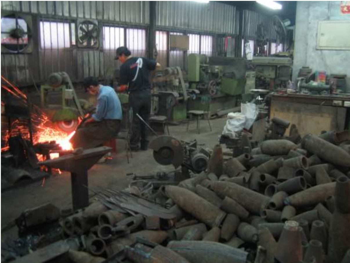
Figure 3 Making the Kinmen Knife amid a dump of artillery shell cases
