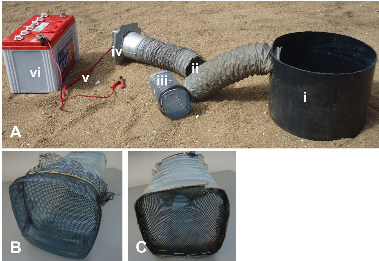
Figure 4. Ovi-ART gravid trap prototype. (A) Trap parts: i) round black bucket, ii) suction tube prepared from collapsible plastic pipe, iii) collection chamber prepared from plastic bottle and fiber glass netting gauze, iv) fan (12V, 0.38A), v) electric cable, vi) 12V battery. (B) Collection chamber backside towards fan. (C) Collection chamber entry funnel.
