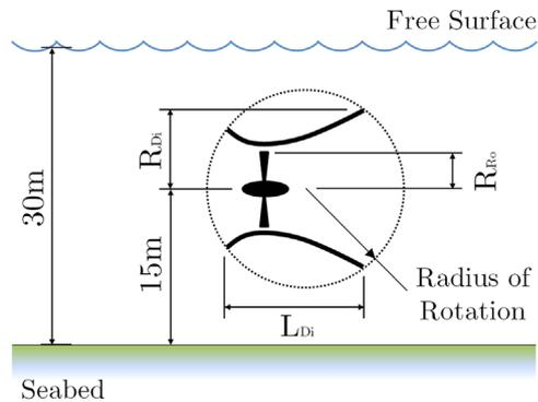
Fig. 3. Tidal channel geometry and optimisation constraints.
