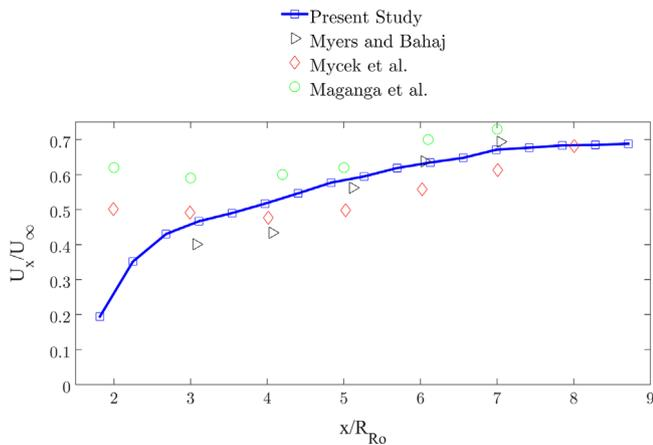
Fig. 14. Normalised velocity for  $-5^\circ$  blade pitch rotor at  $Re=5.5 \times 10^5$ , with a turbulence intensity of 4.7% and tip speed ratio of 5.3, against published data (Maganga et al., 2010; Myers and Bahaj 2010; Mycek et al., 2014).
