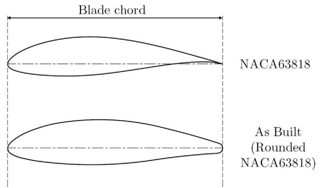
Fig. 1. NACA63818 and as built blade cross sections.
