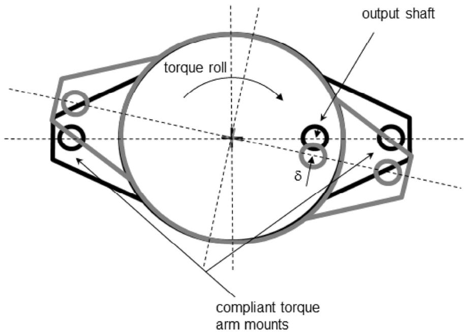
Figure 4 Displacement of gearbox under load induces gearbox-generator misalignment
