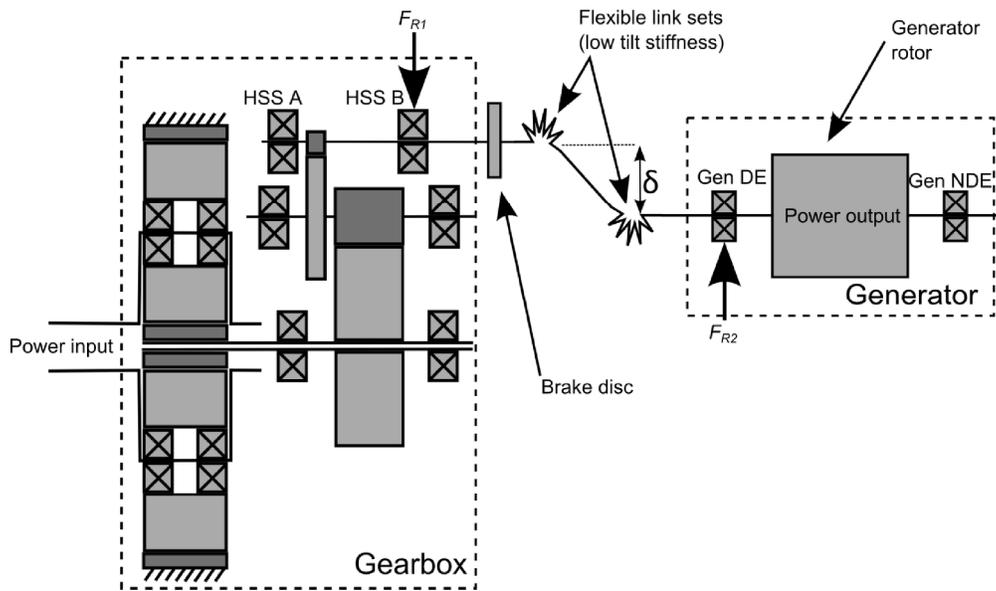
Figure 3 Three stage WT gearbox flexibly coupled to the generator ( $F_{R1}$  and  $F_{R2}$  indicate reaction forces caused by misalignment;  $\delta$  denotes the misalignment)
