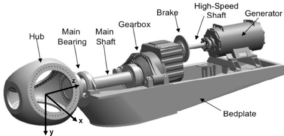
Figure 2 Typical multi-MW WT drivetrain (reproduced from [18], the coordinate system has been added)
