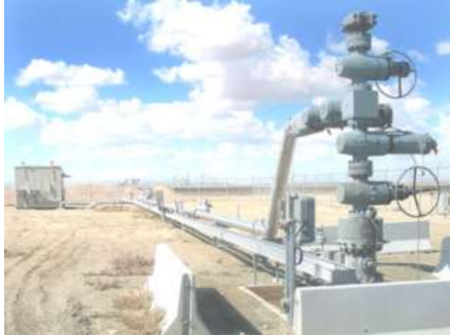
Figure 7. Acid gas injection well at Shute Creek, Wyoming (reproduced with permission from ref. 71).
