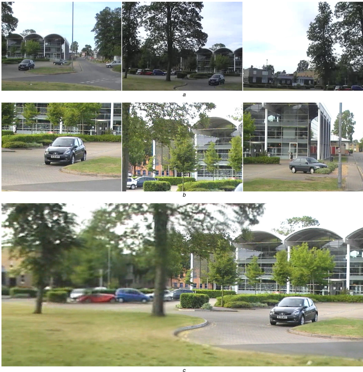
Fig. 1 Video mosaic of varying focal length (resolution) imagery from a PTZ camera a Individual input video frames – without camera Z applied b Individual input video frames – with camera Z applied c The resulting constructed mosaic from input images in ( a ) and ( b )
