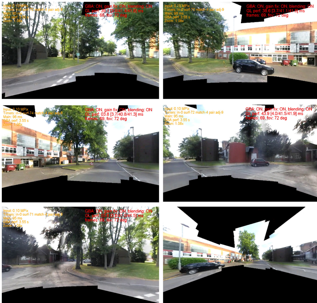
Fig. 11 360° scene mosaic comprising drift-free loop closing
