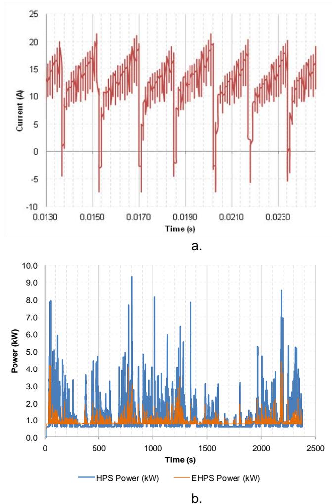
**Fig. 11.** Worst case measured EHPS inverter
