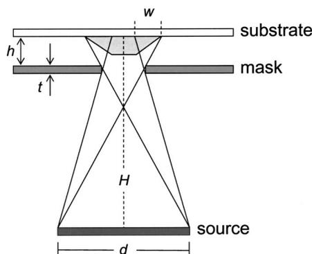
FIG. 3. Factors influencing the sharpness of sidewall features.
