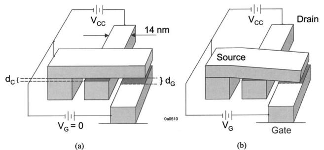
FIG. 1. Vertical nanoelectromechanical switch: (a) Natural open position, and (b) closed position under positive gate bias. As a representative scale, the contact length is chosen to be 14 nm with  $d_C$  and  $d_G$  of 2 and 4 nm, respectively.
