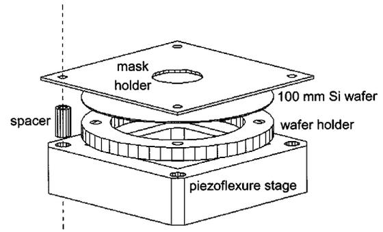
FIG. 4. Fixture assembly for nanotranslated stencil mask and substrate. Parts from top to bottom include: Stencil mask holder, 100 mm Si wafer, wafer holder, spacer, and  $x$ - $y$  flexure nanotranslation stage.
