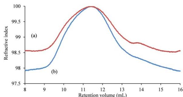
**FIGURE 8** SEC analysis of (a) HEC and (b) HEC treated at 155 °C overnight in presence of 2-amino-2-methyl-1-propanol hydrochloride. [Color figure can be viewed in the online issue, which is available at [wileyonlinelibrary.com](http://wileyonlinelibrary.com).]
