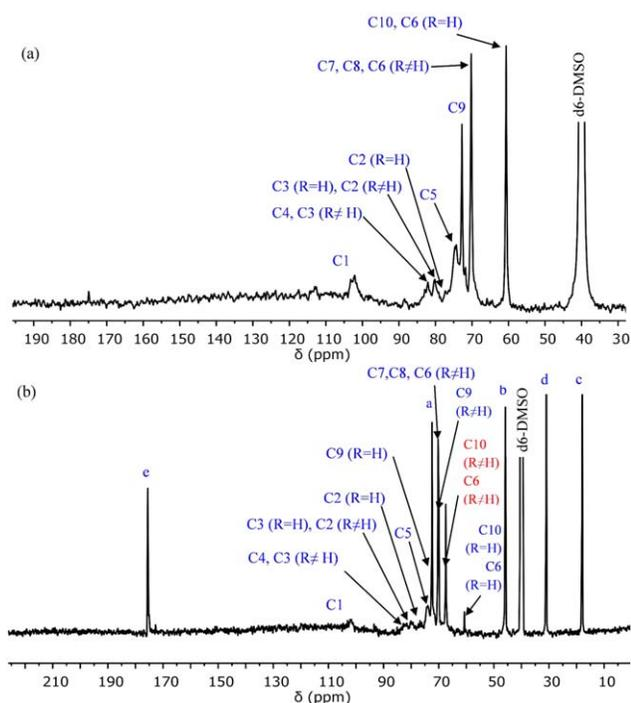
**FIGURE 5**  $^{13}\text{C}$  liquid state NMR (DMSO- $d_6$ , 176 MHz) spectrum of (a) HEC and (b) HMP-functionalized HEC ( $\text{DS}_{\text{primary alcohol}} = 0.9$ ). [Color figure can be viewed in the online issue, which is available at [wileyonlinelibrary.com](http://wileyonlinelibrary.com).]
