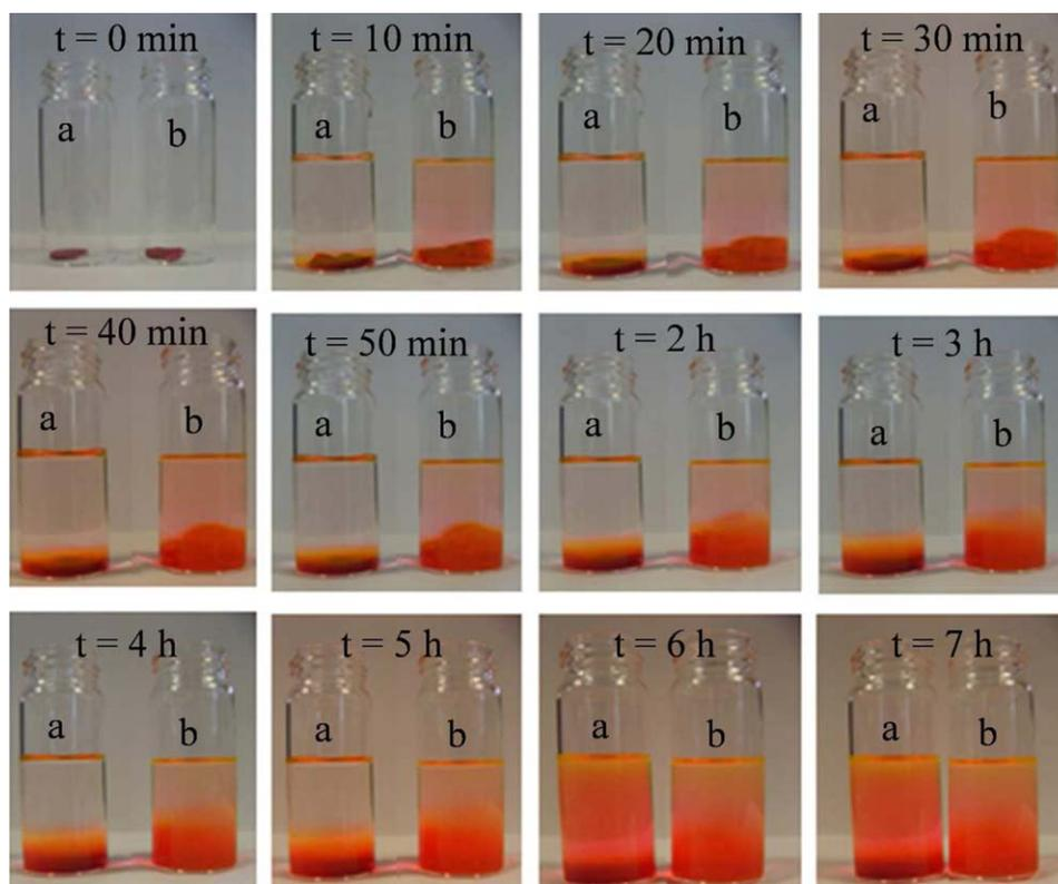
**FIGURE 6** Results of the swelling test of (a) HEC (b) HMP functionalized HEC (DS = 0.9) using rhodamine B. [Color figure can be viewed in the online issue, which is available at [wileyonlinelibrary.com](http://wileyonlinelibrary.com).]
