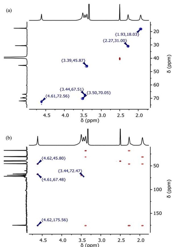
**FIGURE 4**  $^1\text{H}$ - $^{13}\text{C}$  NMR correlation spectra of the HMP-functionalized HEC (a) HSQC (b) HMBC. [Color figure can be viewed in the online issue, which is available at [wileyonlinelibrary.com](http://wileyonlinelibrary.com).]
