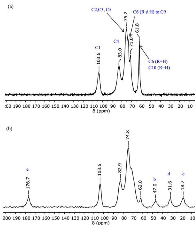
**FIGURE 2** Solid-state MAS CP  $^{13}\text{C}$  NMR spectra of (a) HEC and (b) HMP-functionalized HEC ( $\text{DS}_{\text{primary alcohol}} = 0.9$ ) using cross-polarization (CP) method. [Color figure can be viewed in the online issue, which is available at [wileyonlinelibrary.com](http://wileyonlinelibrary.com).]
