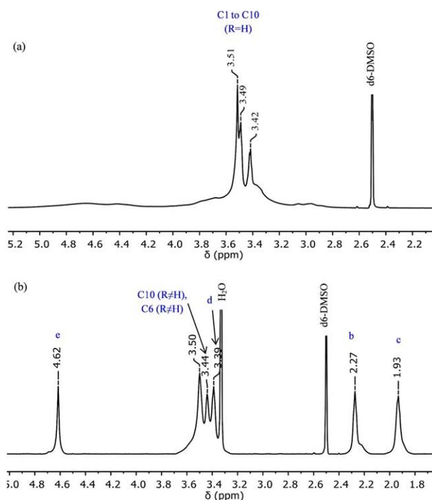
**FIGURE 3**  $^1\text{H}$  NMR spectrum (700 MHz,  $\text{d}_6\text{-DMSO}$ ) of (a) HEC and (b) HMP-functionalized HEC ( $\text{DS}_{\text{primary alcohol}} = 0.9$ ). [Color figure can be viewed in the online issue, which is available at [wileyonlinelibrary.com](http://wileyonlinelibrary.com).]
