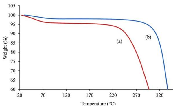
**FIGURE 7** Evolution of weight loss as a function of temperature by TGA (a) HEC; (b) HMP-functionalized HEC ( $DS_{\text{primary alcohol}} = 0.9$ ). [Color figure can be viewed in the online issue, which is available at [wileyonlinelibrary.com](http://wileyonlinelibrary.com).]
