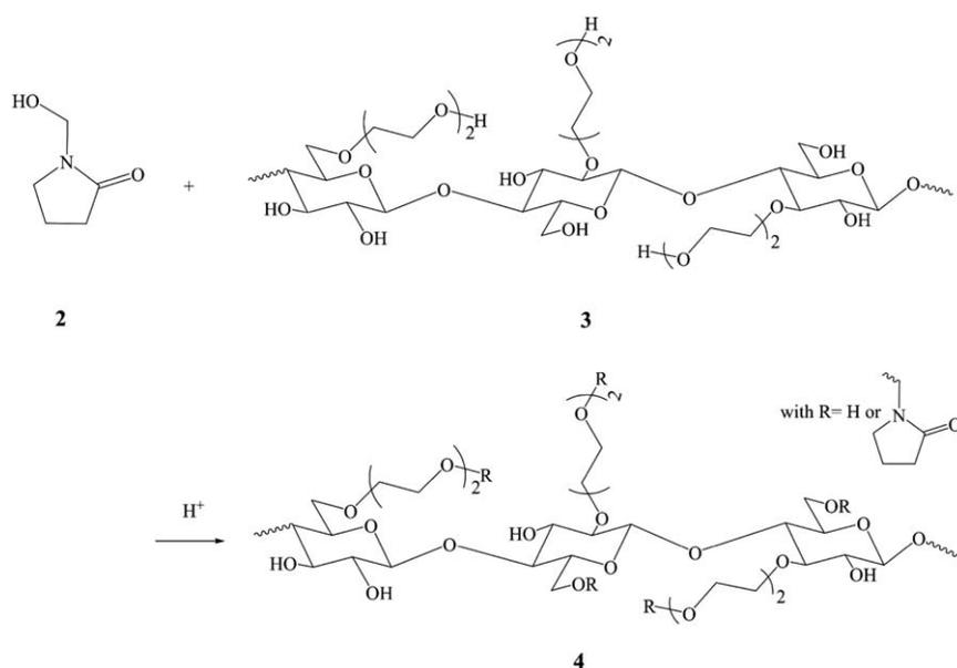
**SCHEME 2** HEC 3 functionalization reaction with HMP 2.
