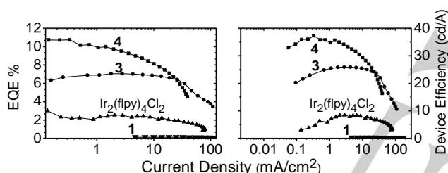
**Figure 4.** Device characteristics for 5% w/w dopant concentration of complexes **1**, **3**, **4** and  $[\text{Ir}(\text{fpy})_2\text{Cl}]_2$ . Data for  $[\text{Ir}(\text{fpy})_2\text{Cl}]_2$  are taken from ref. 25.
