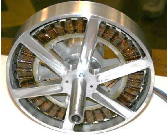
Fig. 1. Prototype motor with compressed aluminum windings.
