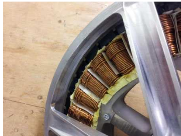
Fig. 8. Front view of the copper wound prototype motor.
