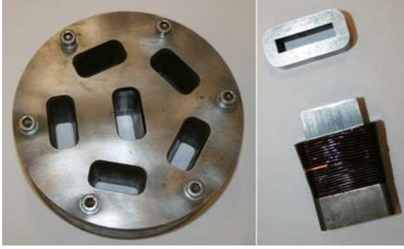
Fig. 3. Compressed winding die (left) suitable for compaction of six coils. Compressed coil fitted to bobbin, pictured with a punch above (right).
