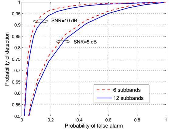
Fig. 4. The performance of  $\text{MS}^3$  for combining Rayleigh faded signals with  $v = 22$  and  $\frac{M}{N} = 0.0219$ , when the received SNR at CRs and the number of subbands change.
