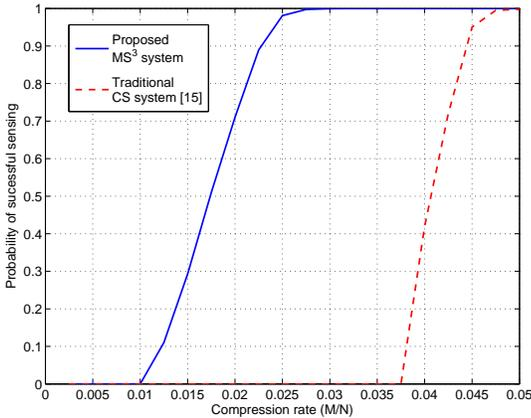
Fig. 6. Comparison between  $MS^3$  and CS-based system [15]. The probability of successful sensing which is defined as the probability of achieving both  $P_d \geq 90\%$  and  $P_f \leq 10\%$ . In simulations, the average SNR as received at CRs is 10 dB and the number of CRs is  $v = 22$ .
