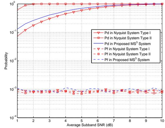
Fig. 5. The probability of detection ( $P_d$ ) and the probability of false alarm ( $P_f$ ) of the proposed  $\text{MS}^3$  system and Nyquist systems over log-normal shadowing channels when the standard deviation  $\sigma = 5$  dB and the average subband SNR varies. In the proposed  $\text{MS}^3$  system, the wideband signal is sampled at different sampling rates by 22 ADCs with the average sampling rate of 448.68 MHz, and the compression rate is  $\frac{M}{N} = 0.0219$ .
