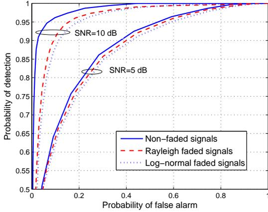
Fig. 3. Receiver operating characteristic curves of  $\text{MS}^3$  for combining non-faded signals or faded signals when the compression rate  $\frac{M}{N} = 0.0219$  and the number of segments  $J = 5$ . The wideband signal is observed by 22 CRs at different sampling rates (the average sampling rate is 448.68 MHz).
