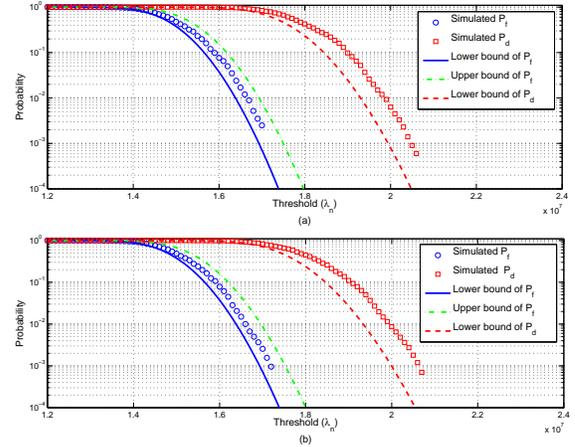
Fig. 2. Comparisons of simulation results and theoretical bounds on the probabilities of false alarm and detection in Theorem 1 and Theorem 2, respectively, when MS<sup>3</sup> combining (a) non-faded signals, (b) Rayleigh faded signals with the received SNR= 5 dB at CRs.
