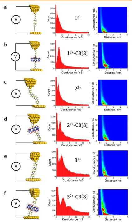
Figure 3. Single molecule conductance measurements: (left column) molecular junction schematic, (center column) 1-D conductance histograms, (right column) 2-D (conductance-junction distance) histograms. The data are for the following junctions  $1^{2+}$  (a),  $1^{2+}$ -CB[8] (b),  $2^{2+}$  (c),  $2^{2+}$ -CB[8] (d),  $3^{2+}$  (e) and  $3^{2+}$ -CB[8] (f).
