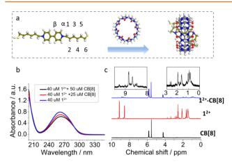
Figure 1. (a) The structure of  $1^{2^+}$  with H atom labeling and complexation with CB[8]; (b) UV/vis spectra of  $1^{2^+}$  with addition of CB[8]; (c) <sup>1</sup>H NMR spectra of CB[8],  $1^{2^+}$ , and  $1^{2^+}$ –CB[8]. The inset is for  $1^{2^+}$ –CB[8]. The left inset shows a magnification of peaks around 9.0 ppm, while the right inset shows magnification of features around 3.0–0.0 ppm.
