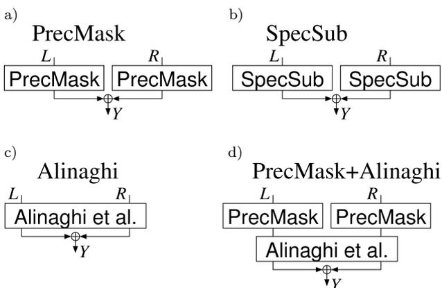
Fig. 4. Block schema of the speech enhancement methods applied prior to ASR.
