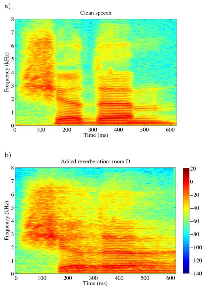
Fig. 1. Spectrograms of the Polish word “siedem” (IPA:  $\text{ɕ} \text{ɛ} \text{d} \text{ɛ} \text{m}$ ), a) close-microphone recording with anechoic BRIR, and b) with 0.89 s reverberation time and 6.12 dB DRR (room D).
