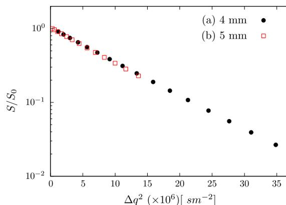
Fig. 2. Calibration of stray field gradient using a sample of water for two different NMR probes. (a) 4 mm probe,  $\Delta = 100 \text{ ms}$ ,  $\delta = 60\text{--}320 \mu\text{s}$ , gradient = 137 G/cm. (b) 5 mm probe,  $\Delta = 80 \text{ ms}$ ,  $\delta = 25\text{--}175 \mu\text{s}$ , gradient = 175 G/cm.
