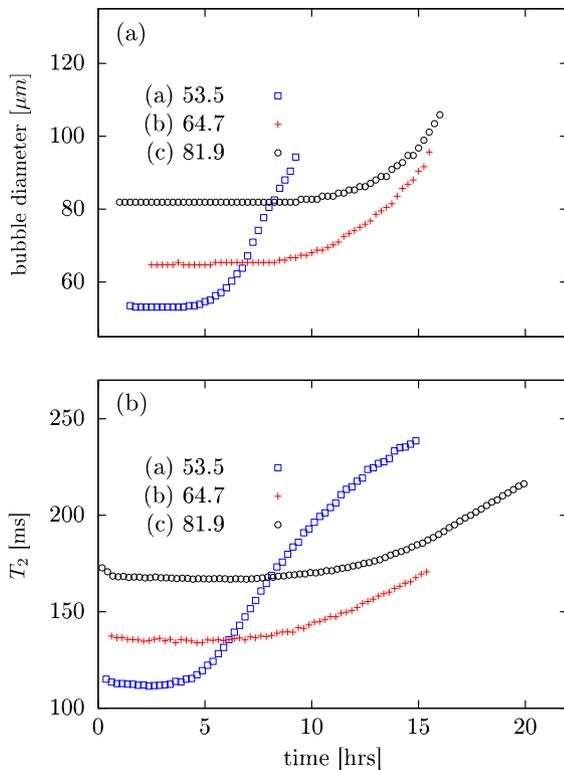
**Fig. 7.** Stability of foam based on the  $q$ -space diffraction NMR data (a) and the  $T_2$  relaxation data (b) for three different initial diameter monodisperse foams. The legend gives the size of bubbles in  $\mu\text{m}$ .
