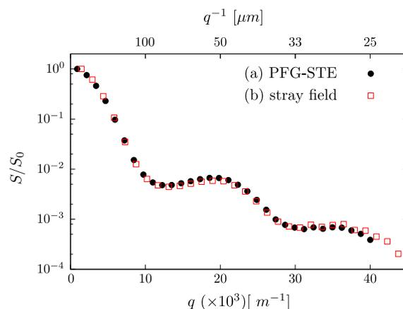
Fig. 3. Self-diffusion NMR experiment of water around 50  $\mu\text{m}$  diameter monodisperse polystyrene beads on a 4 mm probe. (a) PFG-STE experiment,  $\delta = 2 \text{ ms}$ ,  $\Delta = 1 \text{ s}$ . Maximum gradient strength = 50 G/cm. Gradient range from 2 to 90%. (b) Stray-field experiment,  $\delta = 25\text{--}800 \mu\text{s}$ ,  $\Delta = 1 \text{ s}$ . Stray-field gradient = 137 G/cm.
