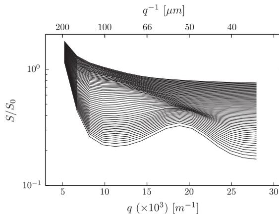
**Fig. 6.**  $q$ -space diffusion data over time for a monodisperse foam sample in a 5 mm NMR tube. Each experimental data set took 15 min to acquire. The foam was monitored for 15 h with the diffraction peak discernible for 8 h. The first acquired data set is at the bottom of the stacked plot.  $\delta = 60$ –320  $\mu\text{s}$ ,  $\Delta = 1$  s. Stray-field gradient = 175 G/cm.
