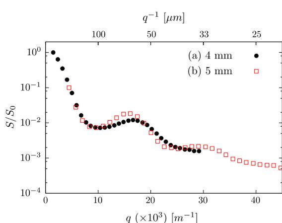
**Fig. 5.** Stray-field stimulated echo CPMG acquisition diffusion  $q$ -space NMR of two monodisperse foam. (a) 4 mm HR-MAS rotor,  $\delta = 25$ –500  $\mu\text{s}$ ,  $\Delta = 1$  s. Stray-field gradient = 137 G/cm. (b) 5 mm NMR tube,  $\delta = 60$ –600  $\mu\text{s}$ ,  $\Delta = 1$  s. Stray-field gradient = 175 G/cm.
