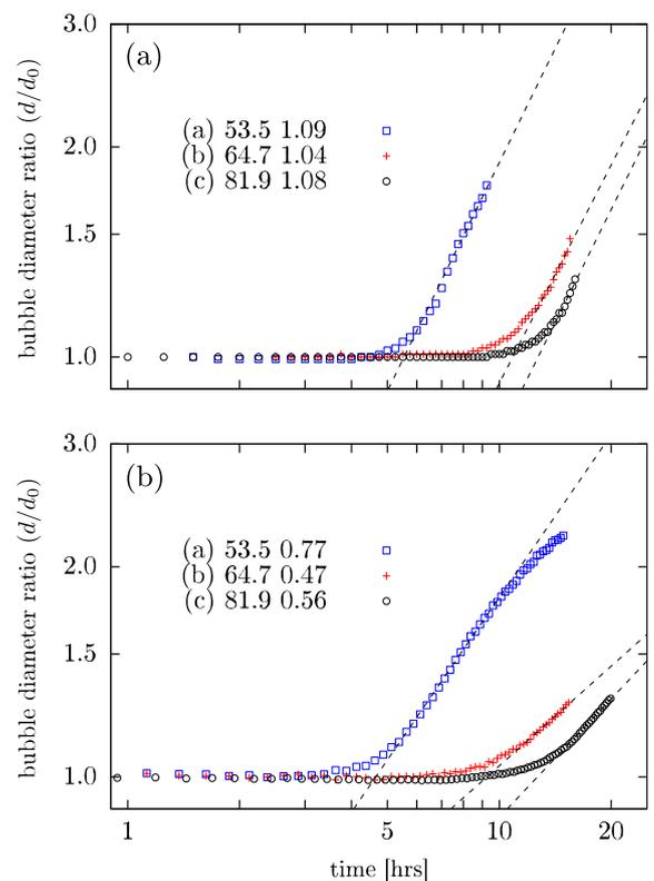
**Fig. 9.** Estimation of the power law coarsening dynamics for three foams of different initial diameters (53.5–81.9  $\mu\text{m}$ ) derived from  $q$ -space imaging data (a) and the  $T_2$  relaxation data (b). The relaxation data has been converted to bubble diameter using the parameters derived from the straight line fit in Fig. 8 the values obtained for the slopes are given in the legends together with the initial bubble diameter.
