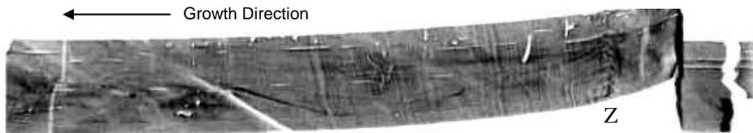
Fig.4.  $0\bar{4}4$  reflection composite image of face C of sample 69-2 formed by summing all images taken at 7.2 second steps across the rocking curve. Image width 35 mm and height 8.5 mm.
