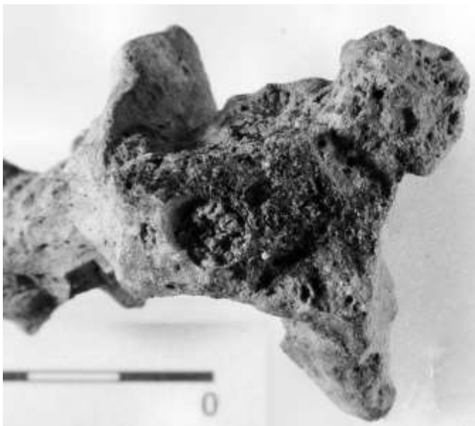
Figure 11: Interior of <Y023> from context (022), showing minute spots of red and green copper alloy in the dark, vesicular FAS matrix.
