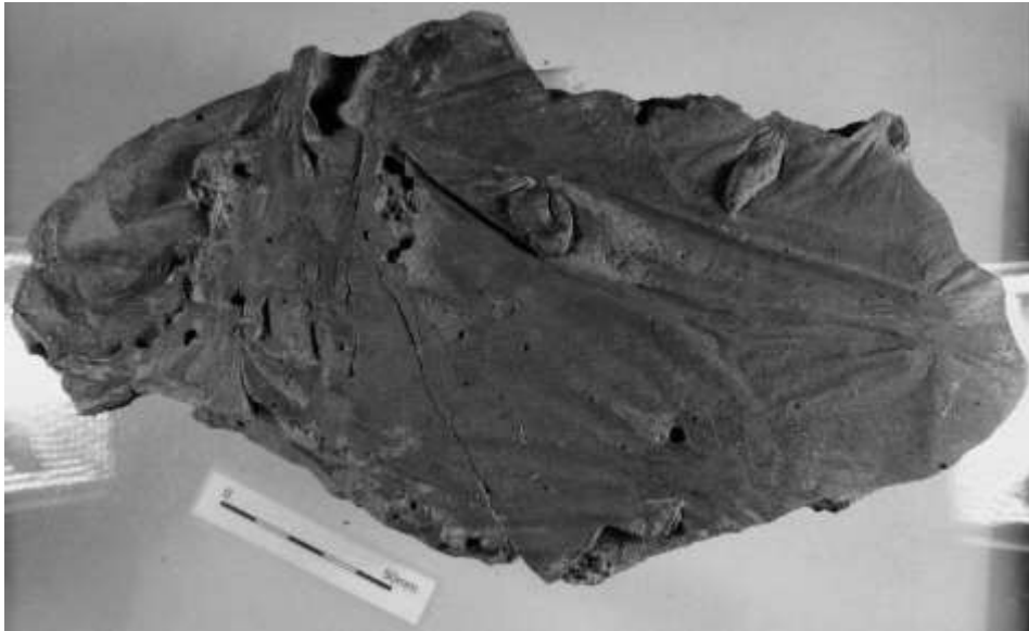
Figure 8: Large broken fragment of iron slag showing smooth dark surface and part of the original curved edge.
