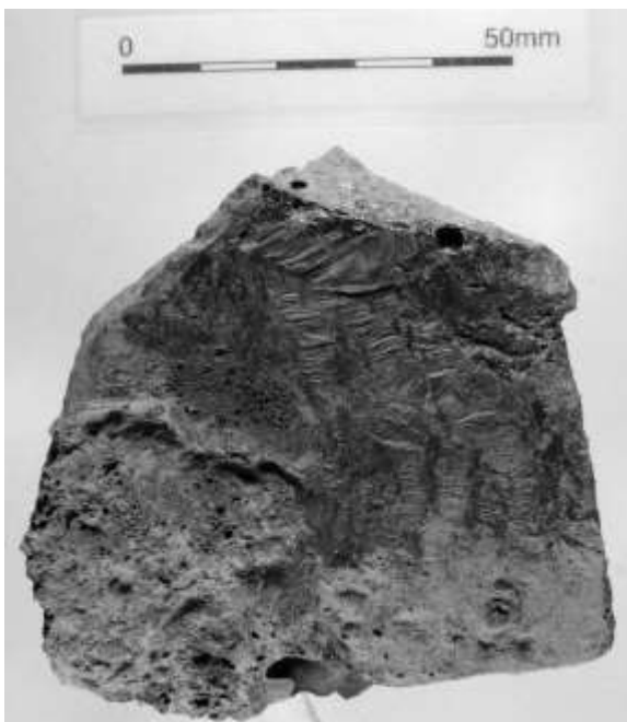
Figure 9: Small fragment of iron slag showing fine surface creasing.
