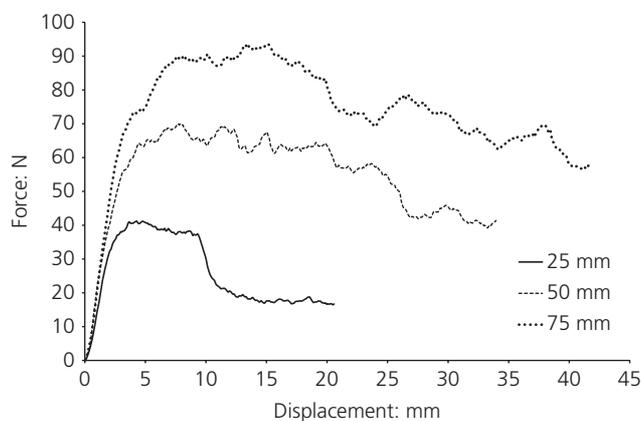
Figure 2. Interface failures for different length fibres (3% WC)
