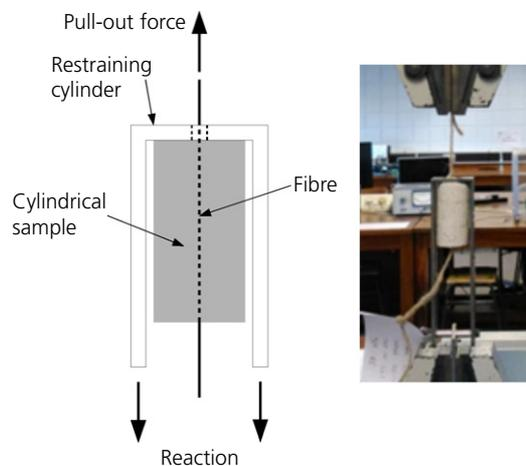
Figure 1. Testing arrangement
