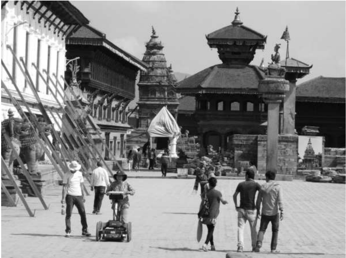
Figure 22: GPR survey being conducted in Bhaktapur's Durbar Square.
