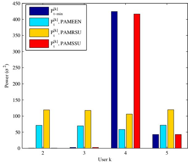
Fig. 10. Transmitted power comparison of SUs with different algorithms of the IA-based CR network in a certain time slot when  $P_t^{max}/K/\sigma^2$  is equal to 20dB.  $R_{th}^{[2]}=0.5$  bits/s/Hz,  $R_{th}^{[3]}=1$  bits/s/Hz,  $R_{th}^{[4]}=5$  bits/s/Hz and  $R_{th}^{[5]}=7.5$  bits/s/Hz.
