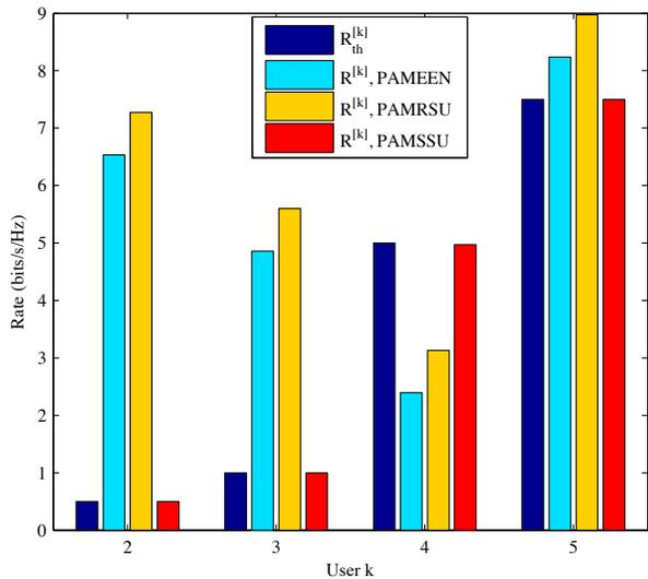
Fig. 11. Rate comparison of SUs with different algorithms of the IA-based CR network in a certain time slot when  $P_t^{max}/K/\sigma^2$  is equal to 20dB.  $R_{th}^{[2]}=0.5$  bits/s/Hz,  $R_{th}^{[3]}=1$  bits/s/Hz,  $R_{th}^{[4]}=5$  bits/s/Hz and  $R_{th}^{[5]}=7.5$  bits/s/Hz.
