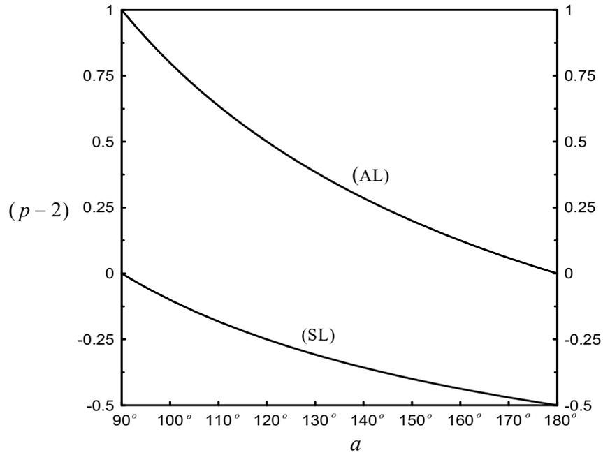
**Fig. 5** Variation of the couple-stress singularity with respect to the angle of the notch  $a$  for symmetric (SL) and antisymmetric (AL) loadings.
