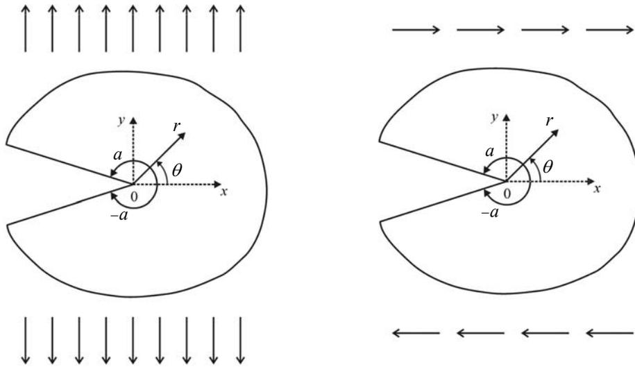
**Fig. 1** Geometry of the elastic notch under plane-strain conditions: (a) Symmetric loading
