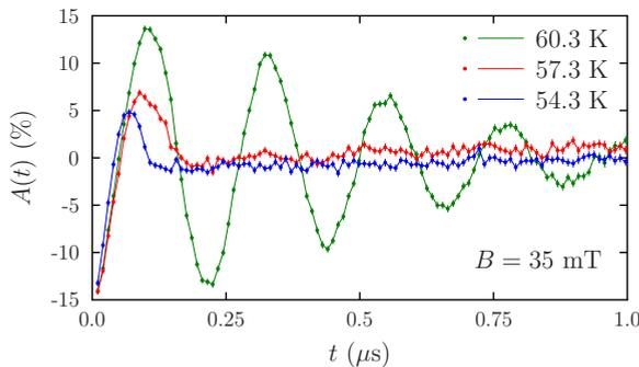
FIG. 3. (Color online) (a) Time-domain spectra measured in an applied transverse magnetic field of 35 mT in the paramagnetic phase at 60.3 K, the skyrmion phase at 57.3 K, and the single- $q$  phase at 54.3 K.
