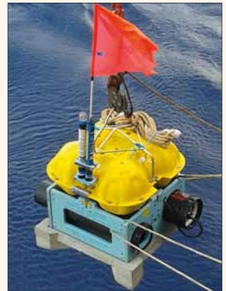
5 An ocean-bottom seismograph (OBS) being launched on JC132. The yellow section contains spherical glass floats; the sensors and data logger are in the box below. The concrete anchor is released on command from the ship to return the instrument to the surface.
