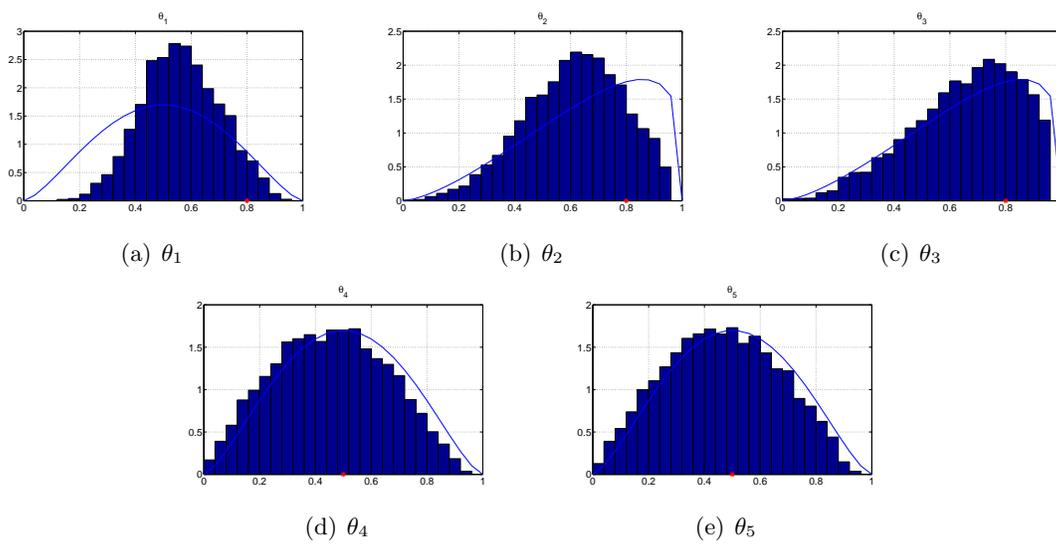
Figure 6: Marginal posterior distributions for the model parameters from the MCMC sample (histograms after 10,000 iterations) along with the prior density (blue curves) using SBGPC.
