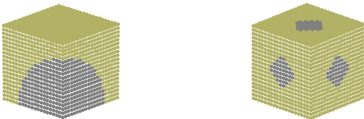
Fig. 7 MPM models for isolated void (left) and connected pore network (right). The black particles are deleted to generate voids.
