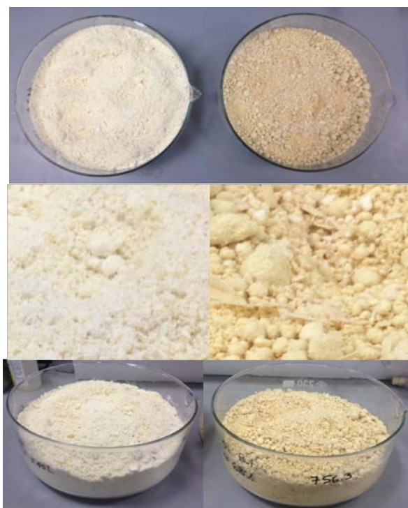
Figure 2. Qualitative comparisons among the particulates produced in flow (left) and in batch (right).
