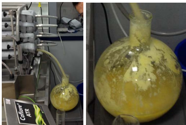
Figure 3. Collection of an analysis sample into a 10 L flask as isolated from the exit port of the first stage reactor.
