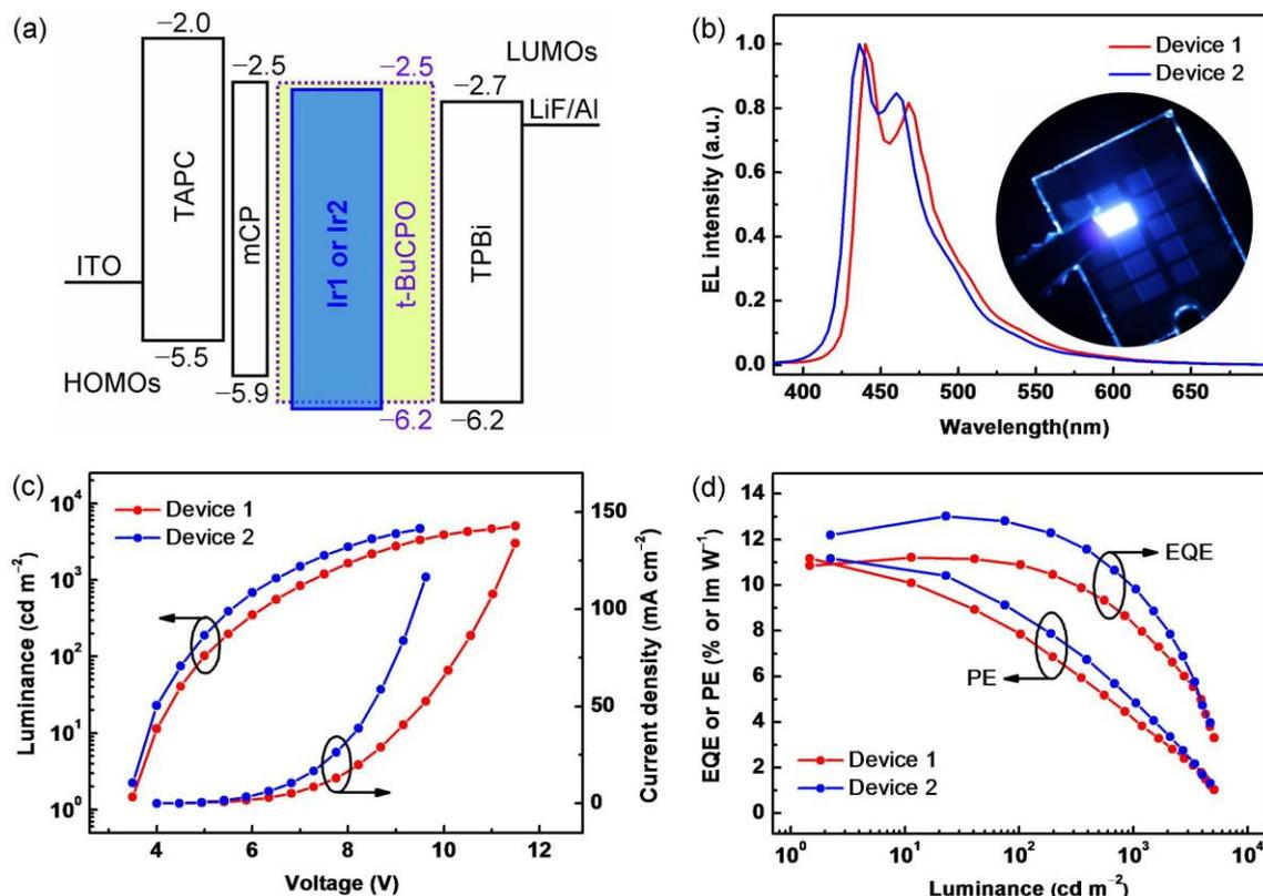
**Figure 3.** (a) Energy diagram of the materials used in the OLEDs. (b) EL spectra of Devices 1 and 2. Inset: a photograph of Device 2 illuminating at 1000  $\text{cd m}^{-2}$ . (c) Current density-voltage-luminance ( $J$ - $V$ - $L$ ) curves of Devices 1 and 2. (d) Power efficiency (PE)-luminance ( $L$ )-external quantum efficiency (EQE) curves of Devices 1 and 2.
