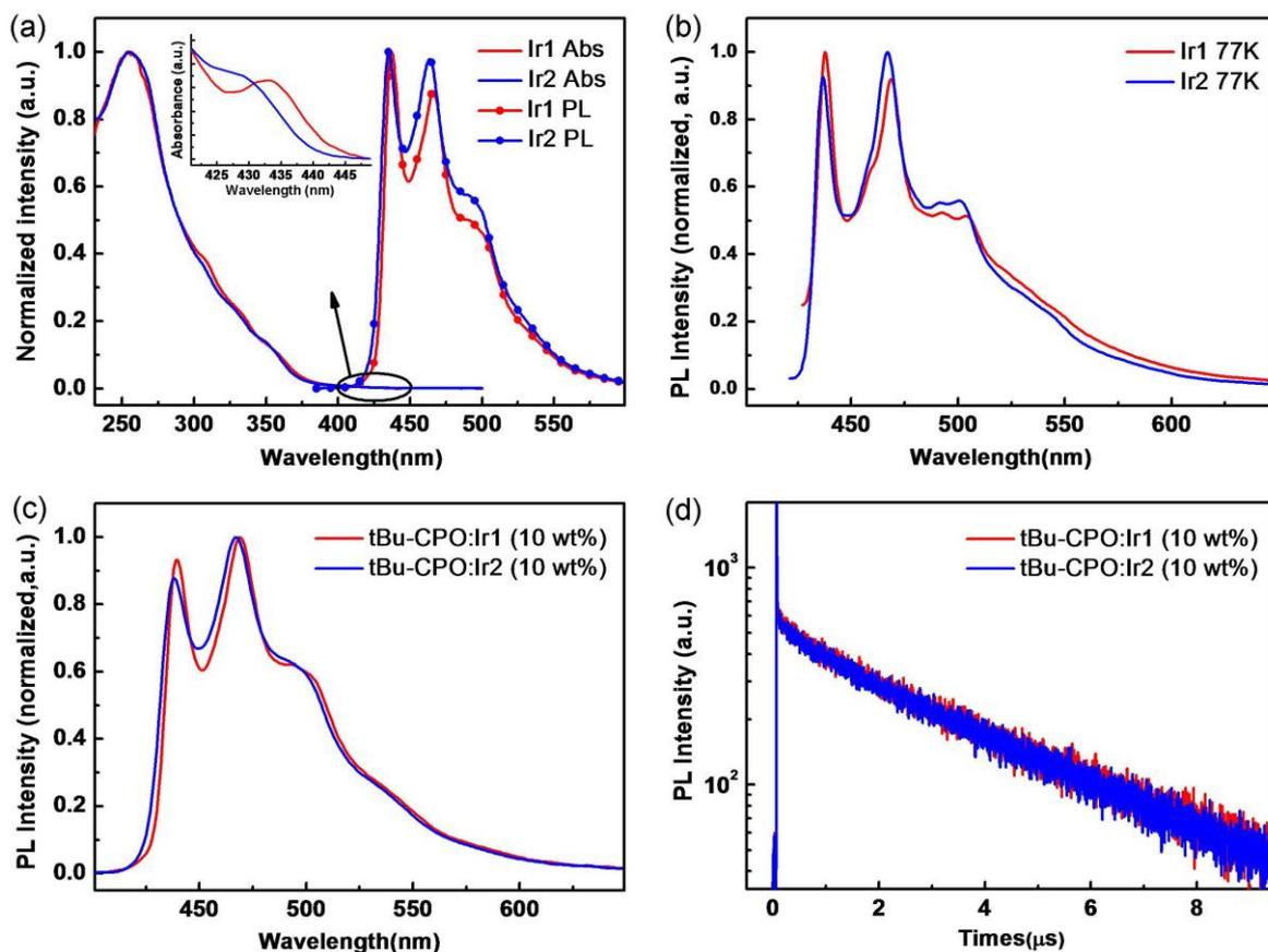
**Figure 2.** UV-vis absorption and PL spectra in CH<sub>2</sub>Cl<sub>2</sub> at room temperature (a) and PL spectra in THF at low temperature (77 K) (b) of **Ir1** and **Ir2**. PL spectra (c) and luminescence decay profiles (d) of tBu-CPO films doped with 10 wt% **Ir1** and **Ir2**. Emission data were obtained in degassed solutions. The structure of tBu-CPO is shown in Figure S3.
