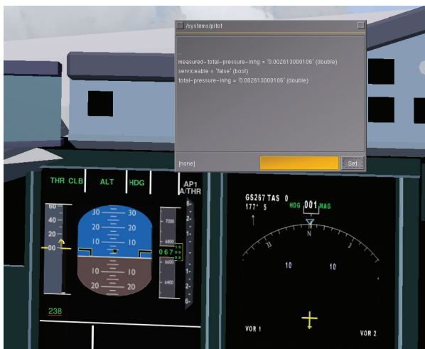
Fig. 3. The effect of hardware pitot fault injection
