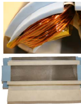
Fig. 9. Upper - End winding of a single tooth coil with a high fill factor – 58% slot fill was achieved. Lower – Single unwound stator segment.
