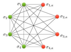
Figure 2. Illustration of the spin graph corresponding to the implementation of the clause  $\sigma_1 \vee \sigma_2 \vee \sigma_3 \vee \sigma_4$ , as well as the parity checking clause  $\sigma_1 \oplus \sigma_2 \oplus \sigma_3 \oplus \sigma_4$ . Logical spin variables are shown as green vertices, ancillae as red vertices, non-zero couplings are shown as black edges and magnetic fields are not shown. Both clauses for OR and XOR only differ in the value of their fields.
