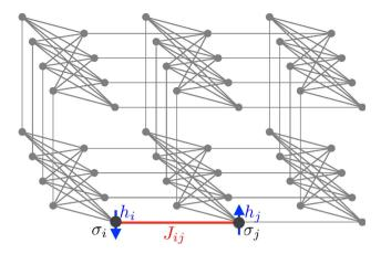
**Figure 1.** A region of a Chimera graph containing  $3 \times 2$  unit cells. Each vertex corresponds to a spin variable. One can adjust the magnetic fields  $h_i$  at each spin as well as the pair-wise couplings  $J_{ij}$  between spins which are adjacent to each other in the graph.
