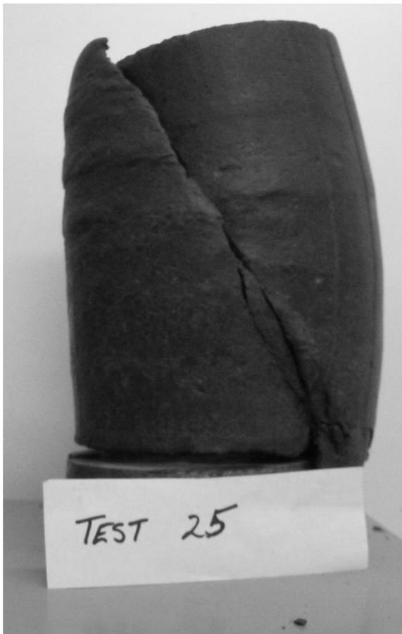
**Figure 24** – Typical shape of failure on samples tested for with  $w_i$  close to 15%.
