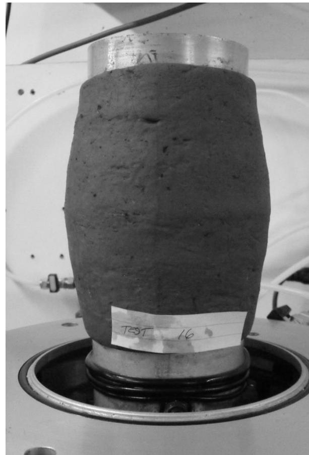
**Figure 25** – Typical shape of failure on samples tested with  $w_i$  close to 20% and 22%.
