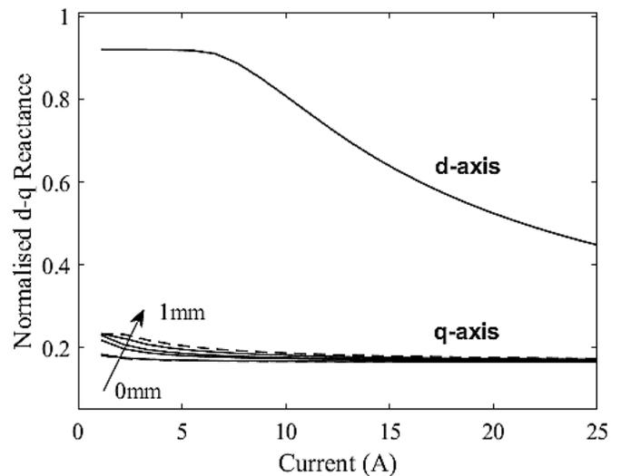
Fig. 10.  $d$ - $q$  Reactance with radial rib thickness
