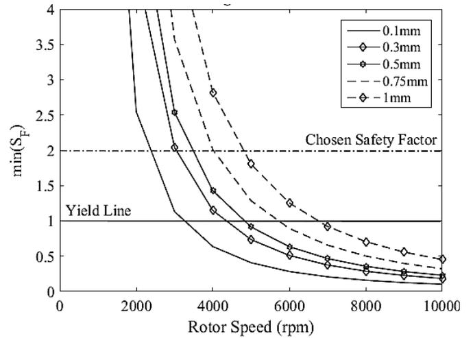
Fig. 14. Minimum safety factor with tangential rib thickness
