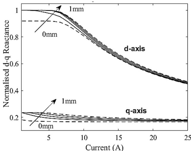
Fig. 8  $d$ - $q$  Reactance with tangential rib thickness
