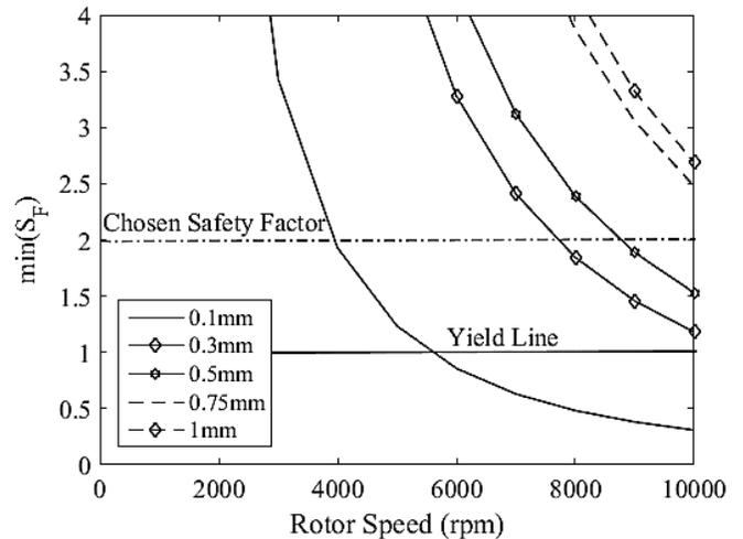
Fig. 16. Minimum safety factor with radial rib thickness
