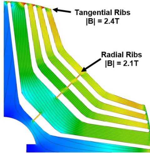
Fig. 6. A and |B| plot showing rib saturation
