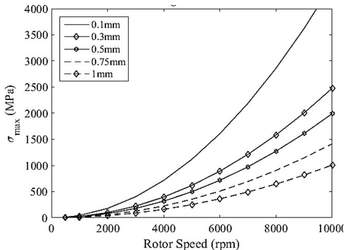
Fig. 13. Peak stress with tangential rib thickness
