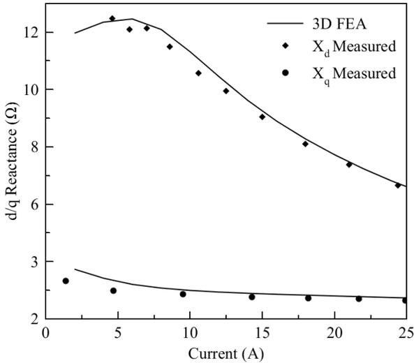
Fig. 5. 3D FEA and Measured orthogonal axis reactance
