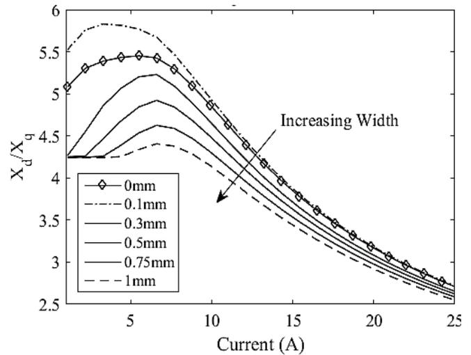
Fig. 9. Machine saliency ratio with tangential rib thickness
