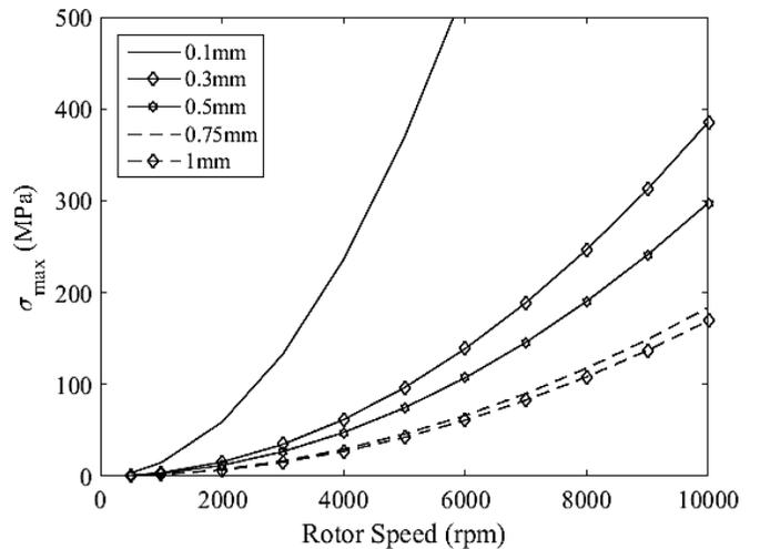
Fig. 15. Peak stress with radial rib thickness
