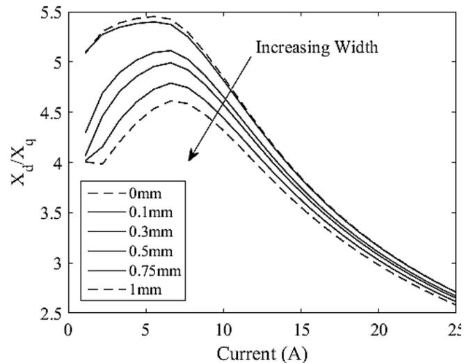
Fig. 11. Machine saliency ratio with radial rib thickness
