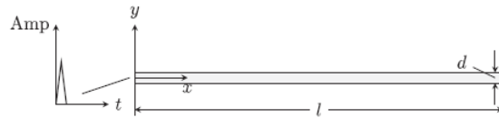
Fig.4 Numerical model used in the FEM simulation.
