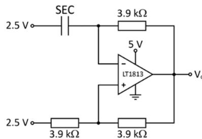
Figure 1. Schematic circuit diagram of the relaxation oscillator.
