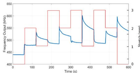
Figure 4: Frequency output of the relaxation oscillator (blue) in response to the SEC being subjected to a stretch pattern (red).
