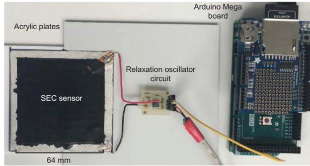
Figure 2. Photograph of the soft elastomeric capacitor based sensor system showing the sensor, the relaxation oscillator circuit and the Arduino microcontroller board.
