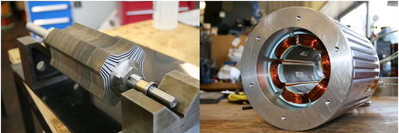
Fig. 11 Rotor (left) and Stator (right) of a prototype cSynRM machine
