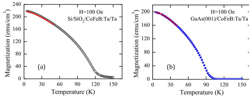
FIG. 1. Temperature dependent magnetization of 100 Å CoFeB:Ta thin-film on (a) Si/SiO<sub>2</sub> and (b) GaAs(001) substrates measured in a 100 Oe applied field in the temperature range from 5 K to 150 K. The red solid lines are the fit curve according to Eq. 1.
