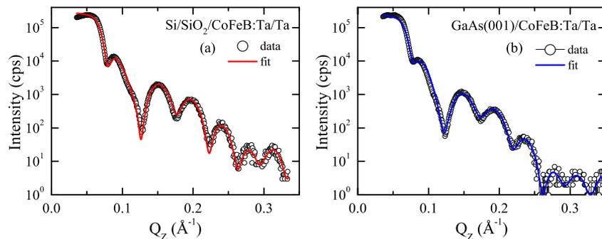
FIG. 2. Specular x-ray reflectivity of CoFeB:Ta thin-films on (a) Si/SiO<sub>2</sub> and (b) GaAs(001) substrates. The solid lines in reflectivity plots are the best fit calculations, using a model which assume that the CoFeB:Ta layer is compositionally uniform.
