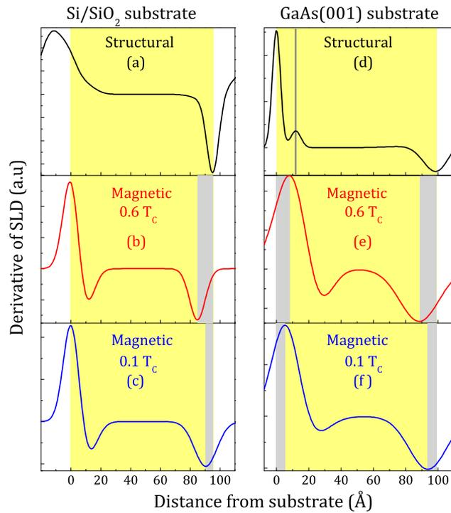
FIG. 5. The derivative of room temperature structural and magnetic SLD profiles for  $0.6 T_c$  and  $0.1 T_c$  to extract layer interfaces are shown for CoFeB:Ta films deposited onto Si/SiO<sub>2</sub> (a-c) and GaAs(001) (d-f) substrates. The vertical dashed lines correspond to the positions of the layer interfaces in the model structures. The shaded regions show magnetic dead layer formations.
