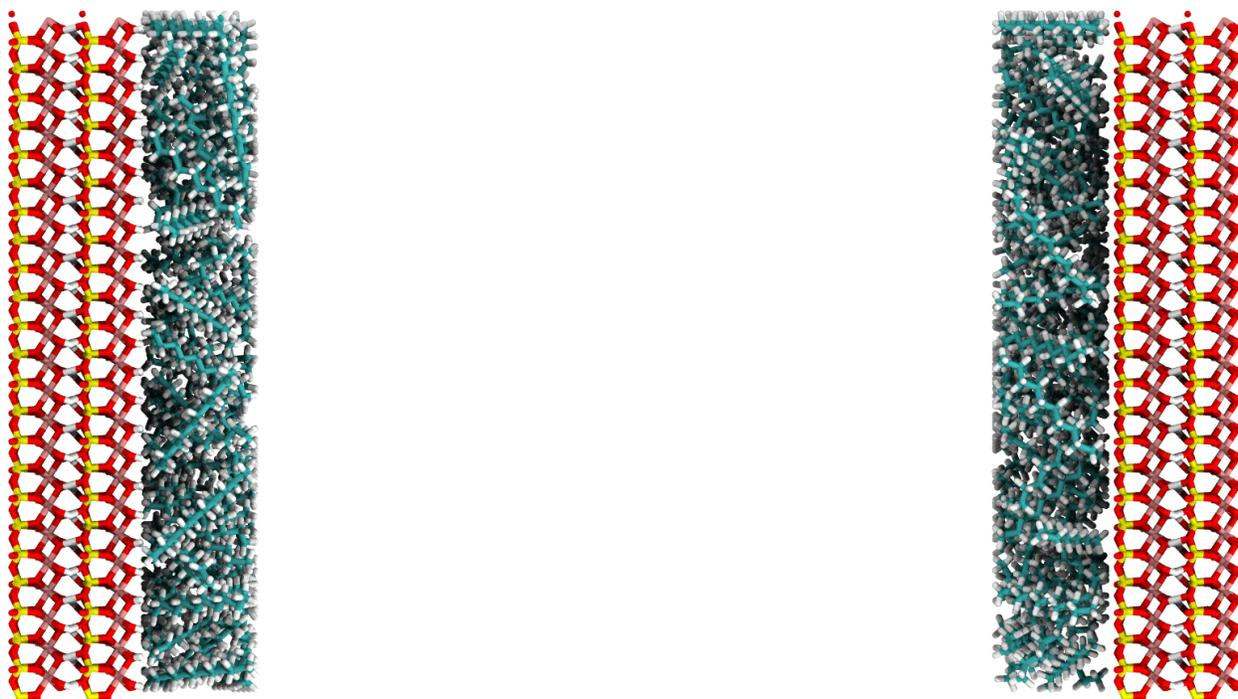
Figure 4: A snapshot showing the initial model of decane interacting with kaolinite before water is added. The PackMol software package<sup>24</sup> has been used to create the densely packed organic phase adjacent to the siloxane and hydroxyl surfaces. All simulations start with similar configurations. The clay structure contains the same color scheme as in Figure 3, whilst the oil molecules contain carbon (blue) and hydrogen (white).
