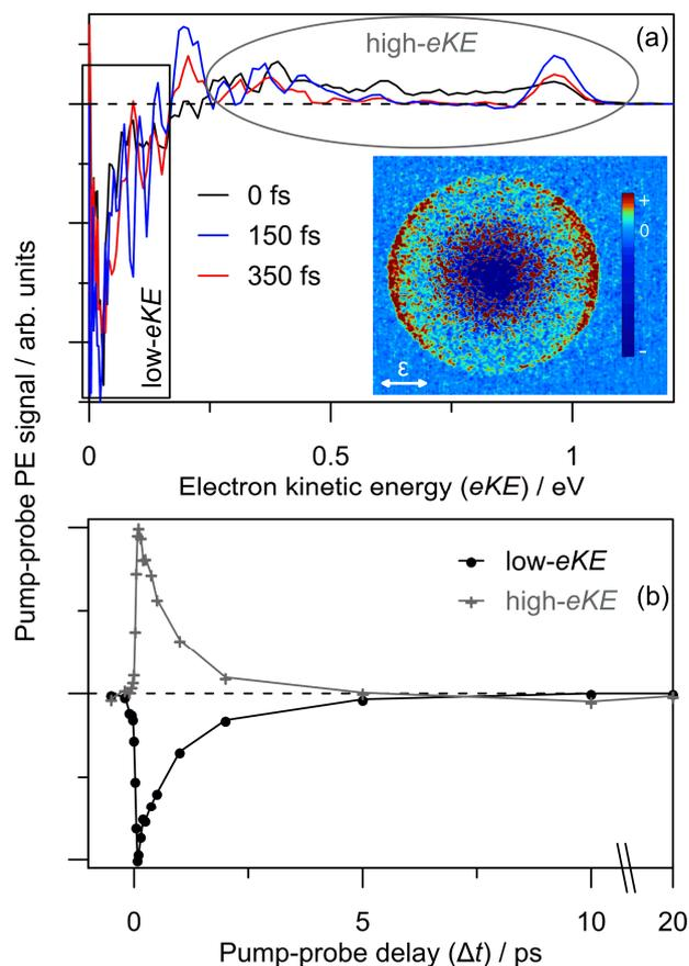
**Fig. 8** 3.10 + 1.05 eV time-resolved dynamics: (a) Three example  $\Delta t$  spectra, which are divided a low- $eKE$  and high- $eKE$  contributions; and (b) integrated contributions of each the two pump-probe contributions. The 150 fs pump-probe velocity-map image is inset in (a), illustrating  $\beta_2 \sim +2$  (relative to the polarisation,  $\epsilon$ ) for the high- $eKE$  feature.
