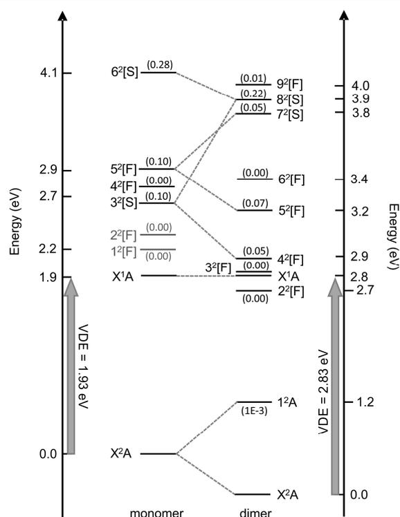
**Fig. 5** Calculated vertical electronic states and  $\pi^*$ -resonances of  $(CQ_0)_2^-$  compared with  $CQ_0^-$  (left, Ref. 28). Oscillator strengths are included in parentheses. The numerical scale indicates vertical electronic energy relative to the ground electronic state ( $X^2A$ ) anion. The DBS is situated  $\sim$ 150 meV below  $X^2A$ .
