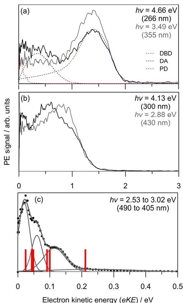
**Fig. 2** Example  $(\text{CQ}_0)_2^-$  photoelectron spectra (black) and  $\text{CQ}_0^-$  (grey) from Ref. 28 at three  $h\nu$ : (a) 4.66 eV; (b) 4.13 eV; (c) average between 2.53 eV to 3.02 eV. Included in (a) are the contributions from the three global-fit channels. The red bars in (c) are calculated carbonyl wagging modes localised on the non-planar monomer.
