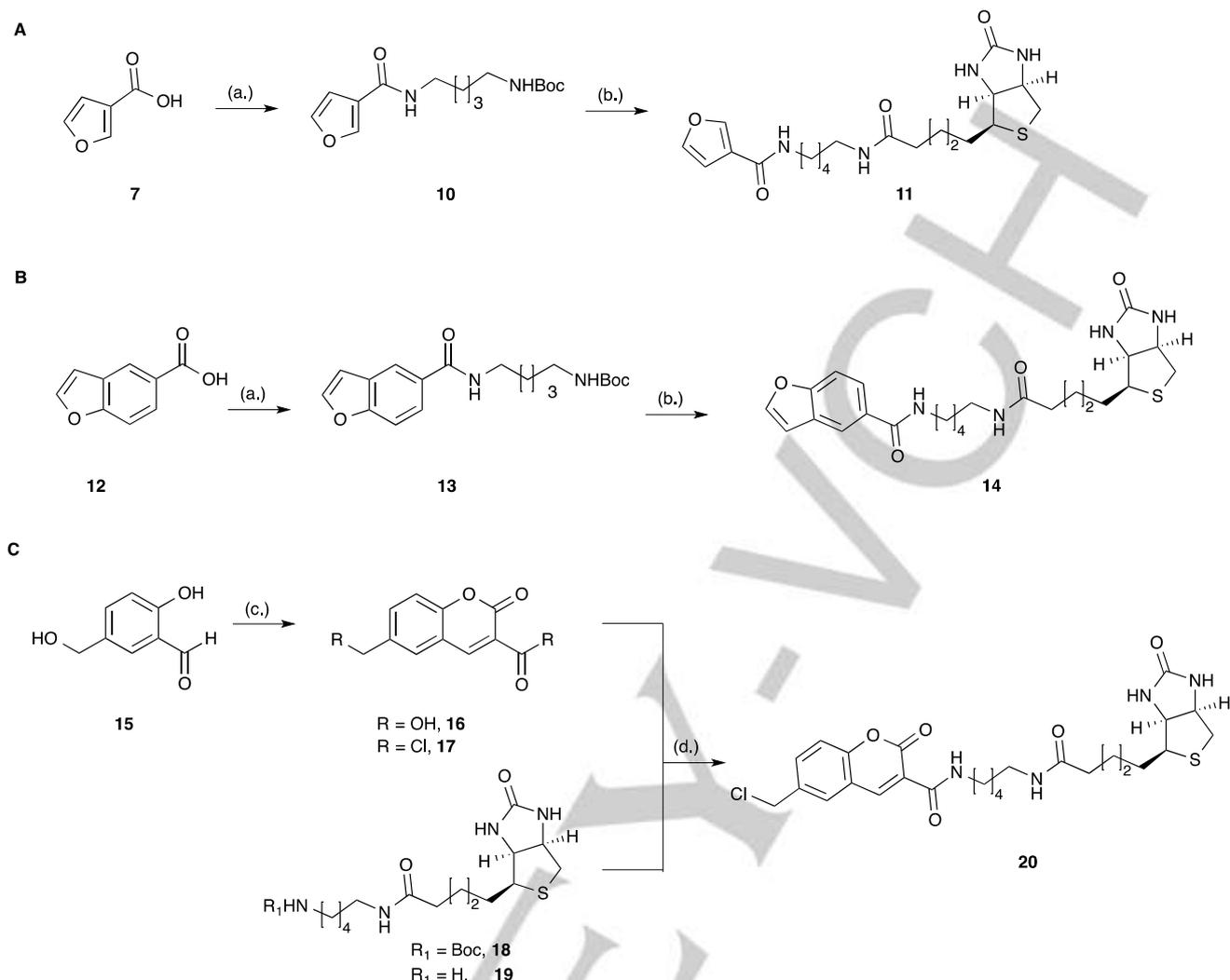
**Scheme 1:** Reagents: (a.) (i.)  $\text{SOCl}_2$ , DMF (cat.); (ii.) N-Boc-1,5-diaminopentane, DIPEA in DCM; (b.) (i.) **10** or **13**, TFA, DCM; (ii.) Biotin-NHS,  $\text{Et}_3\text{N}$ , DMF (c.) Meldrums acid, Pyridine, DCM,  $\Delta$ ; (d.) (i.) **16**,  $\text{SOCl}_2$ ,  $\Delta$ ; (ii.) **18**, TFA, DCM; (iii.) **17** + **19**, *xs.*  $\text{Et}_3\text{N}$
