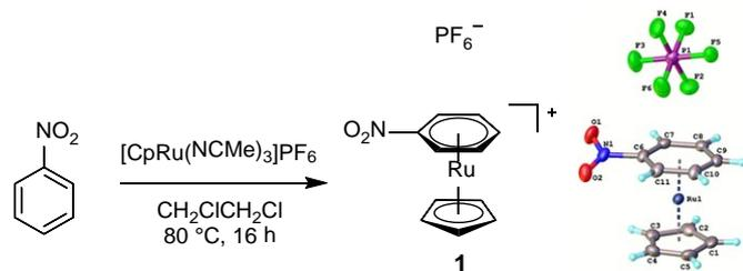
**Figure 1.** Synthesis and molecular structure of complex **1**; thermal ellipsoids are drawn at 50% probability level.
