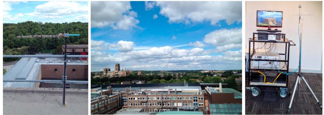
**Figure 7.** Measurement setups: (a) log periodic antenna for 0.25–1 GHz band, (b) antenna view for 0.25–1 GHz band, and (c) indoor setup on trolley for 2.2–2.95 GHz band.
