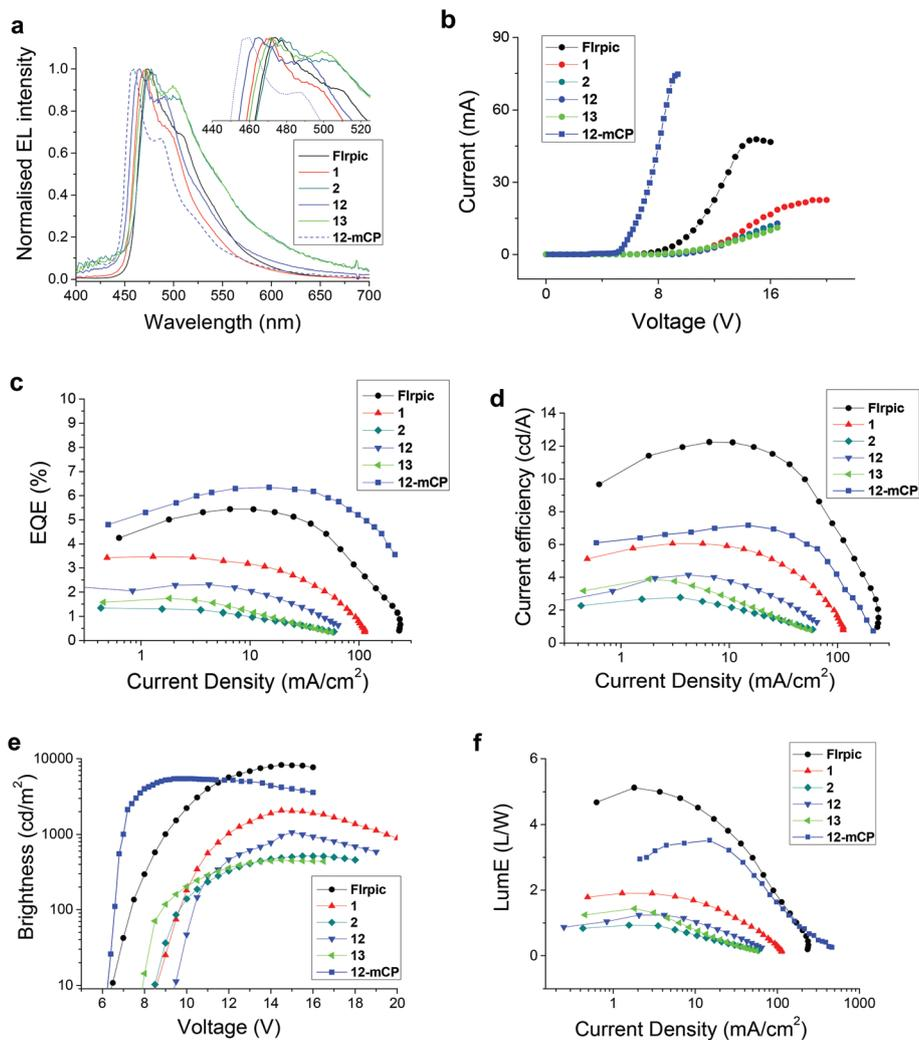
Fig. 6 Electroluminescent device data for complexes Flrpic, 1, 2, 12 and 13 in PVK host and for 12 in mCP host.
