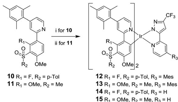
**Scheme 2** Synthesis of complexes **12–15**. Reagents and conditions: i, IrCl<sub>3</sub>·3H<sub>2</sub>O, 2-ethoxyethanol, 130 °C, followed by **9** (for **12** and **13**) or 3-trifluoromethyl-5-(2-pyridyl)pyrazole **16** (for **14** and **15**) DCM/ethanol, 55 °C; ii, [Ir(COD)Cl]<sub>2</sub>, 2-ethoxyethanol, 130 °C, followed by **9** or **16**, DCM/ethanol, 55 °C.
