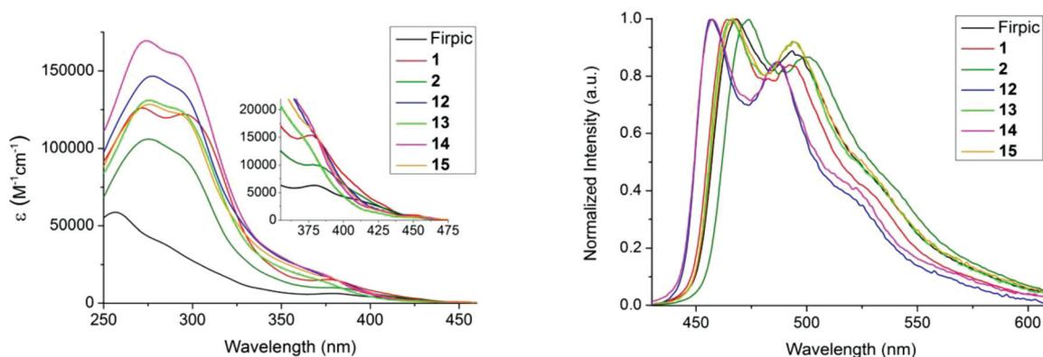
**Fig. 3** (a) UV-Vis absorption spectra of the complexes in DCM [ $<10^{-5}$  M]. Inset shows an expansion of the 350–475 nm region. (b) Emission spectra in deaerated DCM, λ<sub>ex</sub> = 380 nm.
